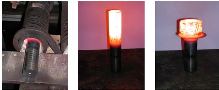
Figure 2: Process stages of preform forming
