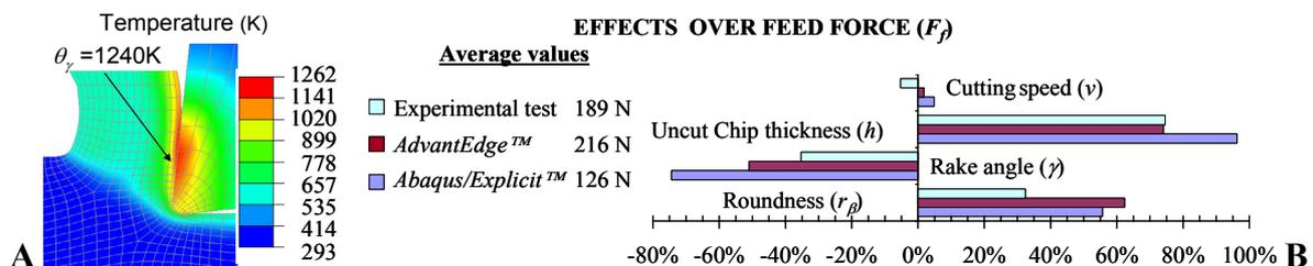
Figure 2: A) Temperature and stress fields (reference values: AISI-4140 steel and P10 insert grade).
