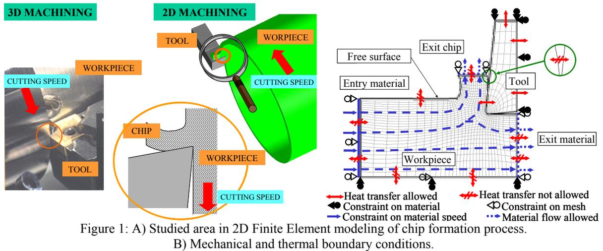
Figure 1: A) Studied area in 2D Finite Element modeling of chip formation process.
