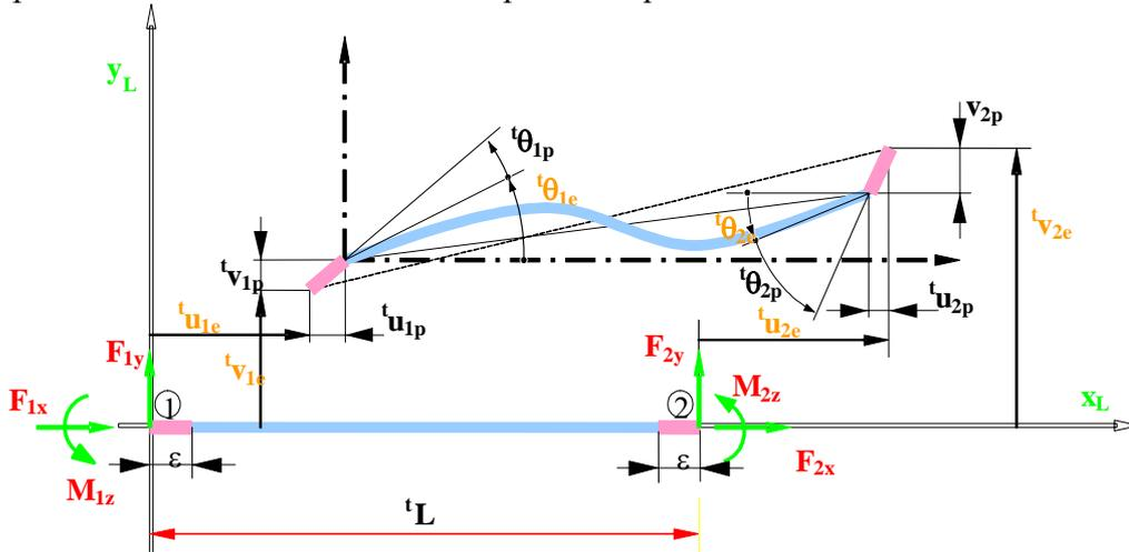
Figure 1: 2D Beam finite element with the possibility of plastic behavior in its ends
