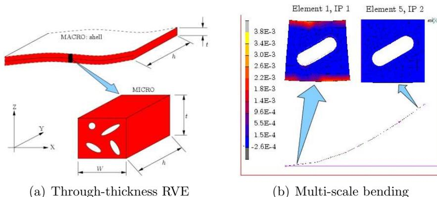
Figure 1: (a) Two-dimensional through-thickness RVE and (b) multi-scale bending of a substructured thin beam
