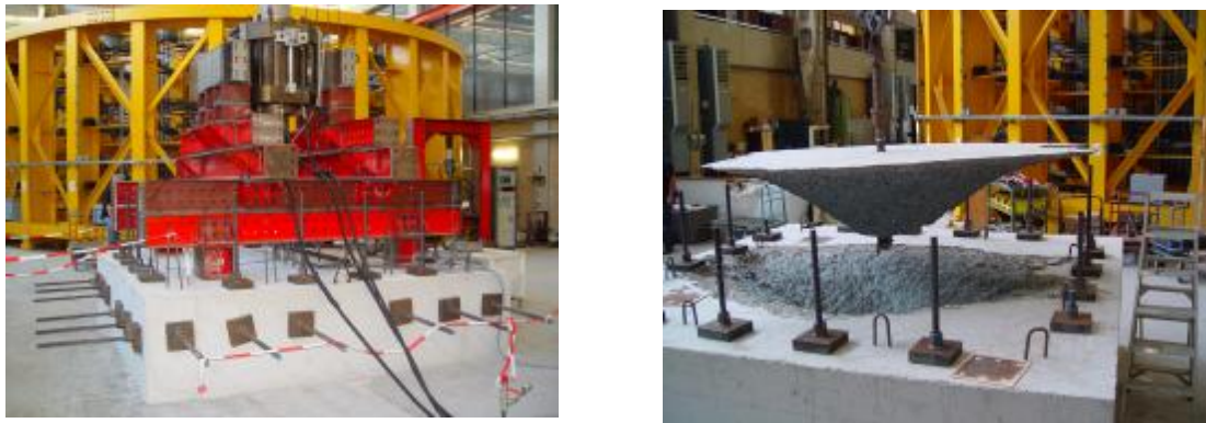
Figure 4 Test set-up + a result of the punching behaviour of the floor with the cone
