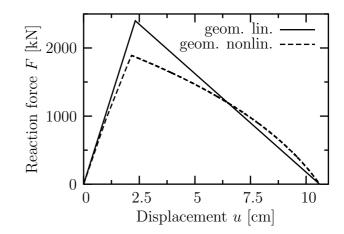
by means of a bifurcation analysis, cf. [5]. According to the snapshot, a typical mode-II failure is predicted. The angle between the normal vector N of the corresponding slip band and the direction of the major principle stress normal is about 45°. By comparing the results obtained from the geometrically linear model with those computed from the finite strain formulation, the importance of accounting for large deformations is apparent.
