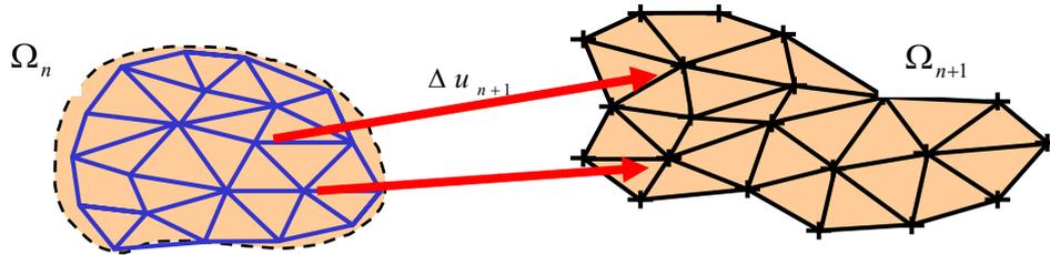
Fig. 2.1 Initial and current configuration and connectivities on the same set of particles
