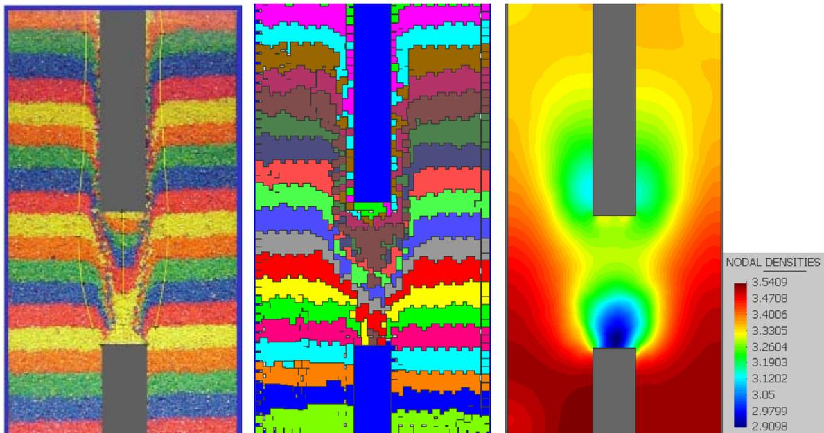
Fig. 3.2 Displacements field and density field after powder transfer stage. Left): experimental distribution of layers after the transfer process, center): numerical distribution of layers and right): density distribution.
