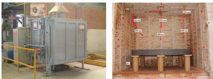
Figure 1: 1m3 furnace (left) and the support grid (right)
