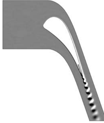
Figure 7. URANS instantaneous span-wise vorticity for 3% case (unsteady, k- \omega )
