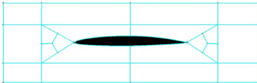
Figure 2 - An illustration of O-grid topology modified with Y-blocks at the leading and trailing edges of the blade.
