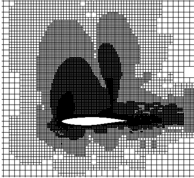
Figure 10: Finest grid obtained after the 5 th refinement cycle for 7 case
