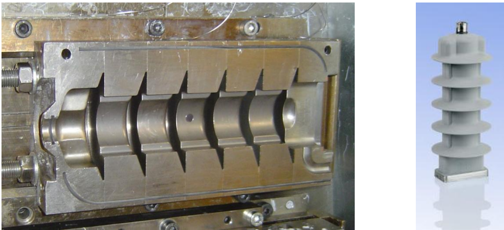
Figure 3: Experimental mold (left) and medium voltage surge arrester (right).
