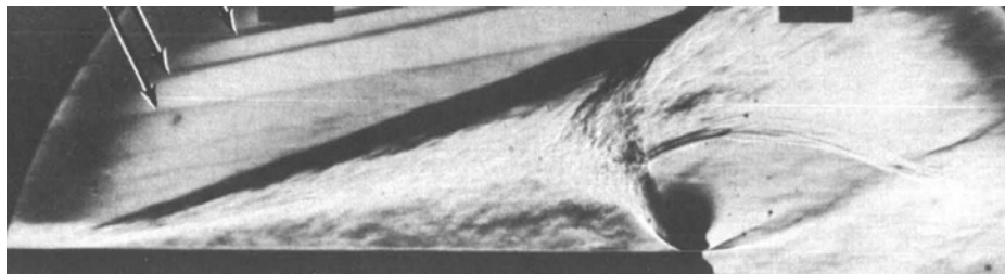
Fig. 5 Computed density gradient of the Case 1 flow (top) and experimental Schlieren photograph 4 (bottom)
