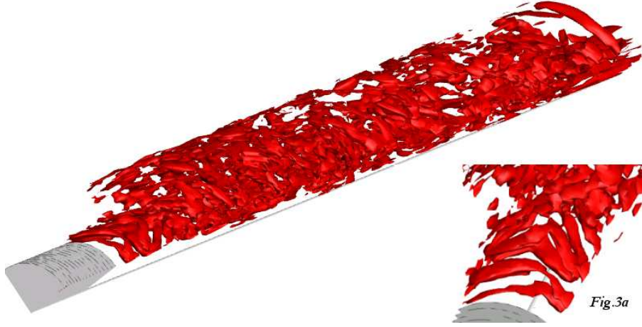
Figure 3: Large Coherent Structure of Axisymmetric Confined Dump Combustor (ACDC) with Q isosurface of 1000
