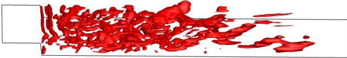
Figure 3: Large Coherent Structure of Axisymmetric Confined Dump Combustor (ACDC) with Q isosurface of 1000
