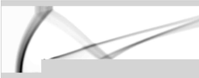
Figure 2: Woodward and Colella [8] forward facing step problem. Mean velocity divergence field. corresponding to an uncertain input Mach number [2.5 : 3.0] . Monte Carlo sampling based on 1000 realizations.
