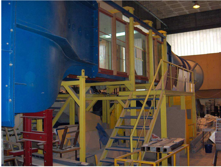
Figure 7. IST's closed-jet wind tunnel.
