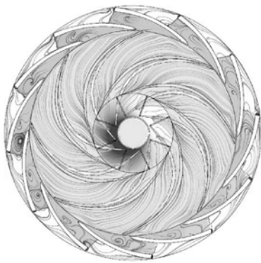
Figure 15: Stream lines of the flow at 1150rpm and 20m 3 /h, notice the differences between the rotor and diffuser.
