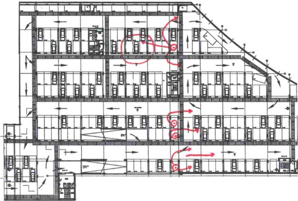
Figure 5: Flow pattern in the tests of fire detection zone 2.
