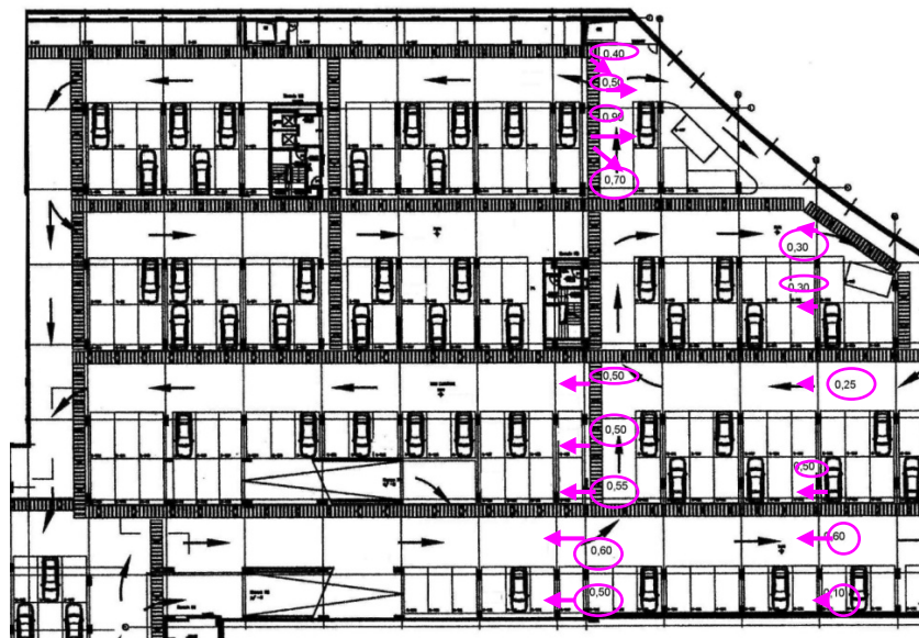
Figure 4: Measured velocities and directions for fire detection zone 1.
