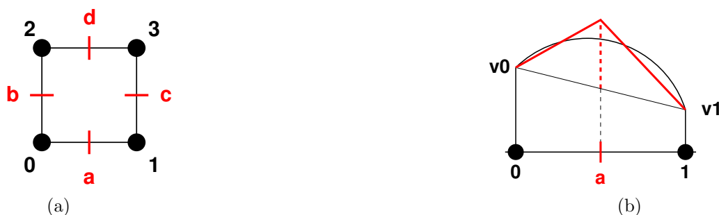
Figure 4: Additional DoF \tilde{u}_i, \tilde{v}_i on cell faces: (a) locations and directions; (b) example representation of \tilde{v}_a (dashed red line) as hierarchical surplus with identical integral value as the parabola to approximate.
