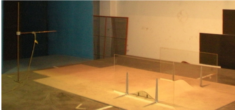
Figure 7: Wind tunnel working chamber and pile setup.
