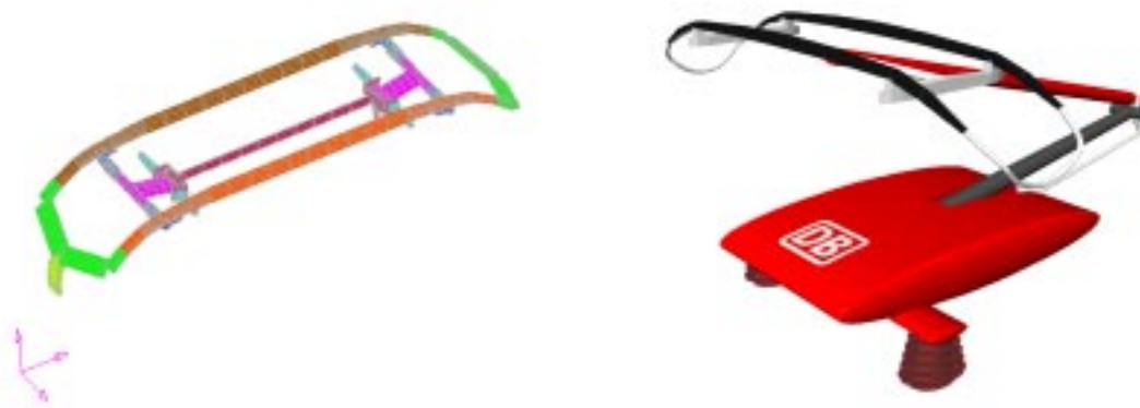
Figure 4: Aero-acoustically optimised pantograph out of ADtranz-DB collaboration.
