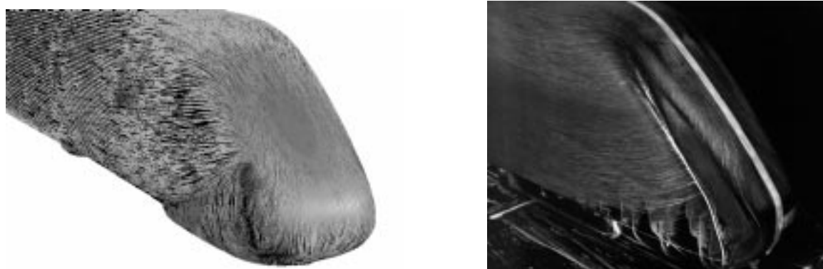
Figure 9: Wall flow pattern on the surface of the trailing vehicle (CFD-calculation 1:1 and model scale 1:7)
