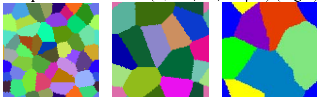
Figure 1: Different initial microstructures applied in the CA model in which each grain has its own orientation ( \theta ).
