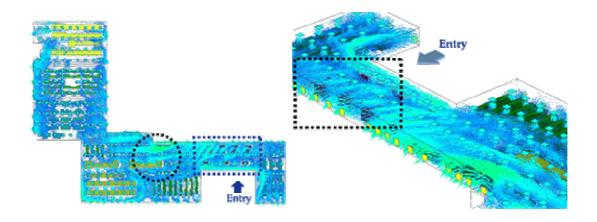
Figure. 1 The overview of flow pattern (Left: Top View, Right: Zoom near Entry)
