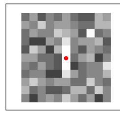
Figure: Average moduli map of 10 morphologies with extreme Von Mises stress at the test point (red circle). Whiter colors represent higher modulus. Higher local stresses at x show a strip like configuration of stiff material B.
