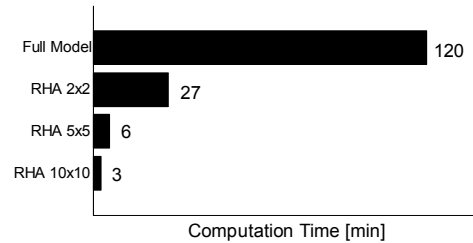
Fig. 6 Computation times of the full model and RHA models on a 3GHz processor. In this case, the computation time can be reduced by a factor of 40.
