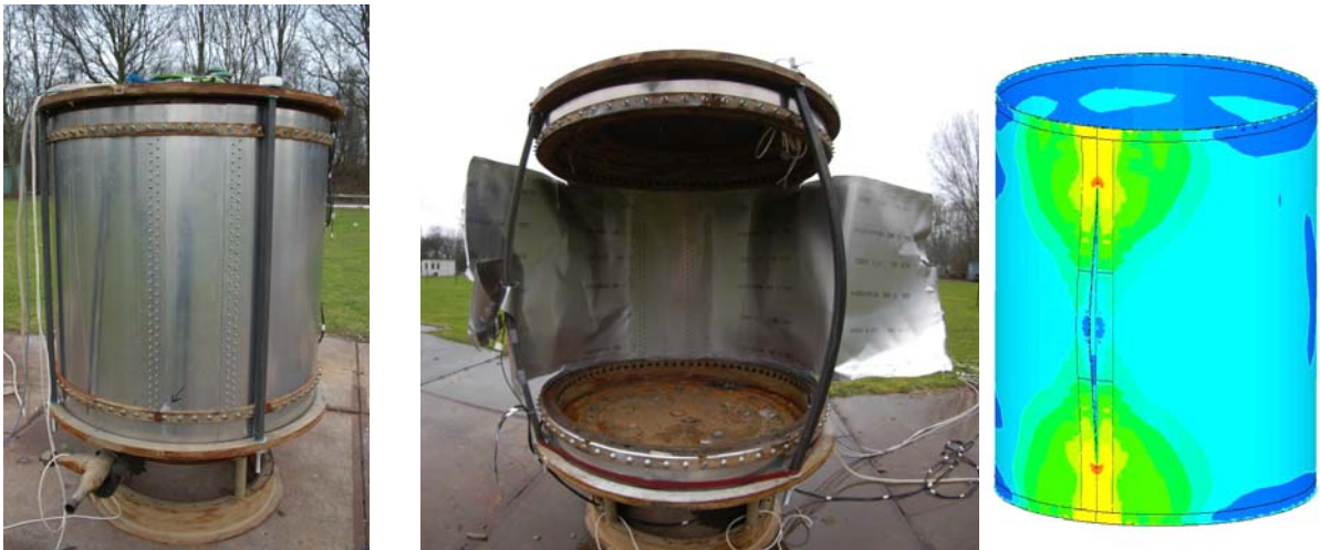
Figure 2 Failure of an pressurized aluminum barrel. (left) setup with measuring devices, (middle) barrel after explosion; (right) FE model, stress field during crack propagation.
