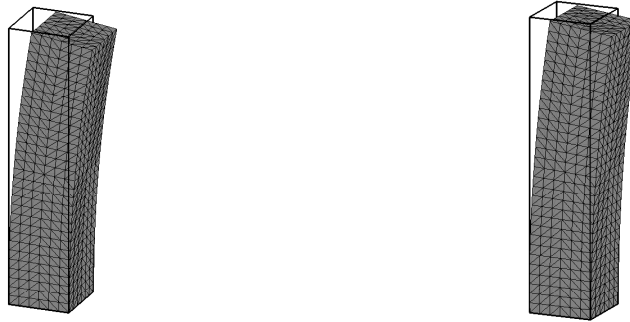
Figure 1: Reference configuration and displacement field at initial time (left) and after 66 days (right).
