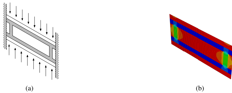
Figure 2: Generalized plane strain model of a masonry cell (a). Out-of-plane stresses in the brick and in the mortar (b).
