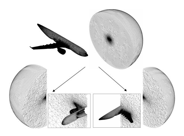
Figure 1: Domain partitioning using Delaunay-based technique.
