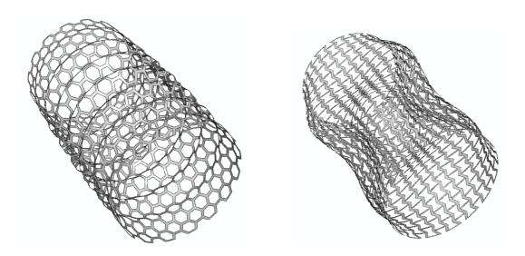
Fig. 1 Buckling modes of an axially compressed lattice cylinder having a regular hexagonal (left) and a standard auxetic topology (right).
