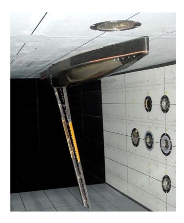
Figure 2: Half model used to investigate the effect of the peniche under high Reynolds number conditions.
