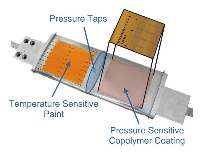
Figure 1 : FLIRET 2D model for pretest in the ETW pilot facility which was used for roughness investigations.
