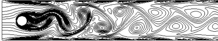
Figure 2. Vorticity of a low Reynolds number flow ( Re = 100 ).
