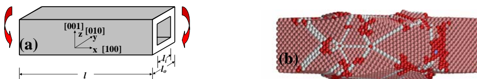
Fig. 1. (a) The geometry of copper nanowires and (b) the formation of two conjoint fivefold deformation twins. The atoms in pink, white and blue are those in local fcc, hcp and icosahedral lattices, respectively; while disordered atoms in red represent surfaces and dislocation cores.
