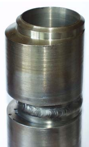
Fig. 2. Tubular type instrument (flux-tube) for heat flux measurement
