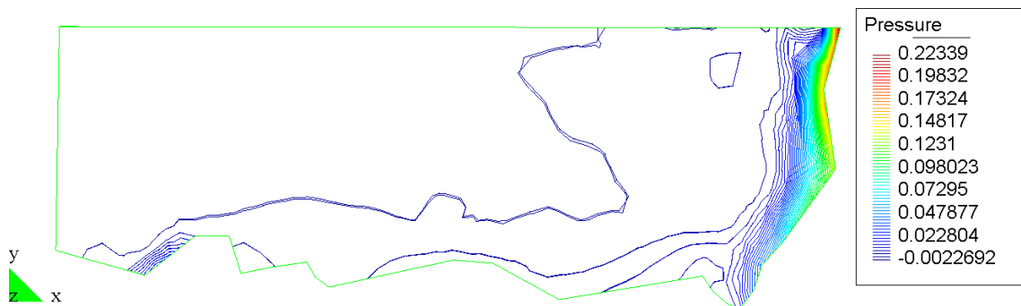
Figure 2: Non-hydrostatic pressure fields
