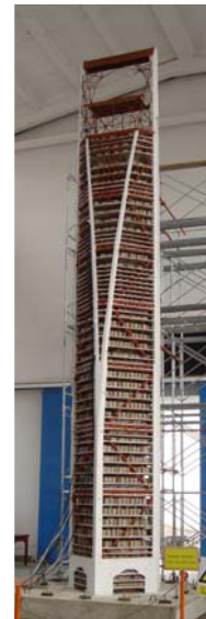
Fig.1 a test model of a super tall building structure built in China
