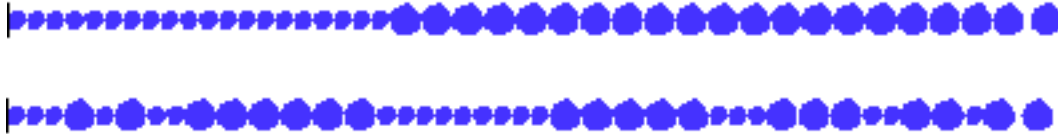
Fig. 1: Initial ( top ) and optimal ( bottom ) configurations of a two-radii granular chain subject to an impact with a striker ( rightmost particle ).
