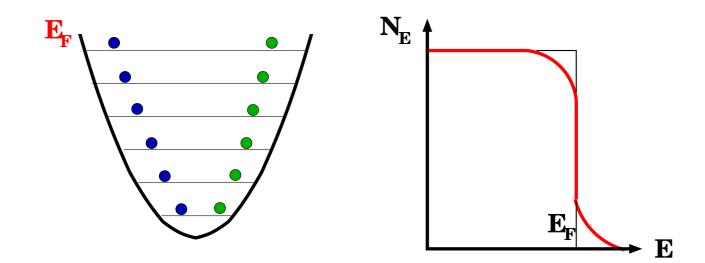
$$E_F = \frac{\hbar^2 k_F^2}{2m}; \quad k_F = (3\pi^2 n)^{1/3}; \quad E_F \sim N^{1/3} \hbar \omega$$
